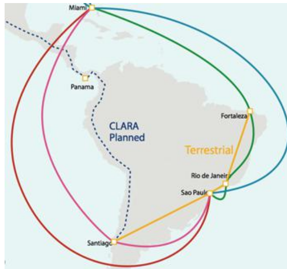
Fig. 1. AmLight topology connecting Miami in the U.S., Fortaleza, Rio de Janeiro and São Paulo in Brazil, and Santiago in Chile. AmLight also operates circuits from Panama City to Miami in a collaboration with RedCLARA.
